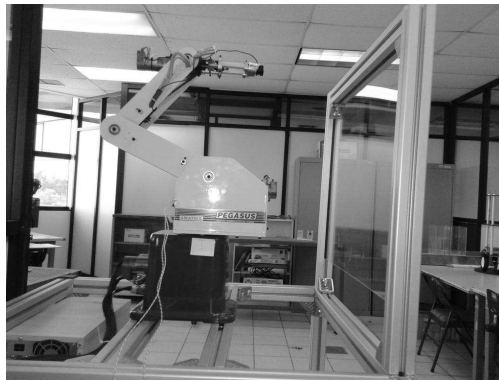
Fig. 2. Pegasus robot configured to have a position constraint.
